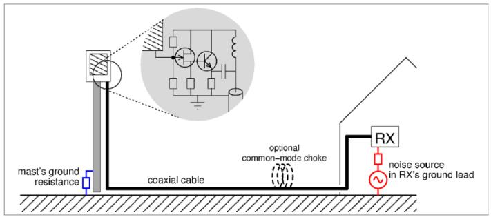
The figure shows a typical MiniWhip setup. At the left is a mast carrying the actual MiniWhip, consisting of a metal plate and an amplifier. The mast is grounded, but that grounding is not perfect, as illustrated by the blue resistor. At the right is the indoors receiver. Indoors, there are often noise sources, such as noise on the mains grounding. These are represented here by the red voltage source, which causes the ground connection of the receiver to not be purely at ground potential.
